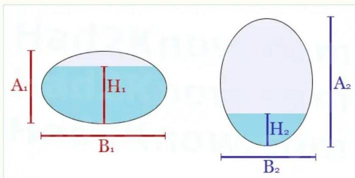
If the height of the tank is **A**, the width of the tank **B**, and the height of the elliptical segment **h** then the area of the segment is given by the equation:
